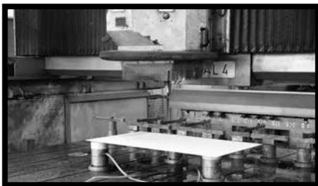
**Fig.24** - All versions of SLIMTECH can be cut with CNC machines. Cutter rotation speed ranges from 12000 to 18000 RPM. The cutter must be pushed forward at a speed ranging from 0,5 to 1 m/min.
