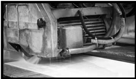
**Fig.23** - All versions of SLIMTECH can be cut with diamond discs. Use discs made especially for porcelain stoneware and in good working order. Disc rotation speed must be high (>2000 RPM) and speed at which tool is pushed low (from 0,5 to 1 m/min.) Depending on the type of disc and the length of the cut, it may be necessary to cool the disc with water.
