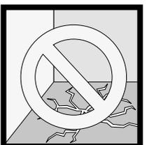
**Fig.37** - In cement-based screeds, the presence of cracks due to hygrometric shrinkage is caused by one or more of the following factors: too much water in the mixture, too fine a grain size of the aggregates, too much cement. Before installation, seal any cracks and holes.
