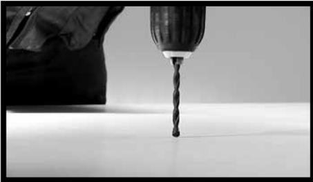
**Fig.16** - As far as manual drilling is concerned, use tungsten bits with a diameter up to 10 mm, fitted to electric drills or battery-operated screwdrivers.
