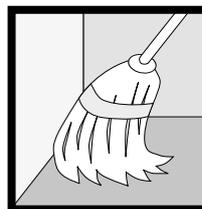
**Fig.36** - The support must be clean. Dust, oil, grease, dirt and debris must be removed as they may compromise adhesion of the adhesive.
