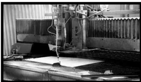
**Fig.25** - All versions of SLIMTECH can be cut with water jet cutting machines. Adopt a speed ranging from 2 to 3 m/min.
